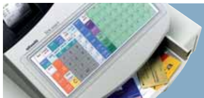
Customizable keyboard, with 42 PLU key and direct selection of up to 126 articles
